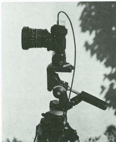
Figure 1: Pentax LX 35mm camera with a 28mm perspective correction lens; shown on a tripod with a cable release.
